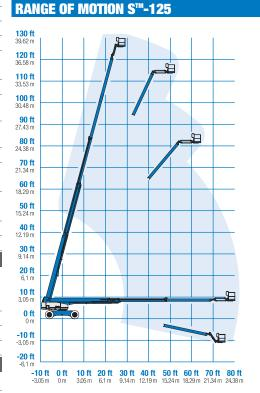
$<sup>^{\</sup>star}$  The metric equivalent of working height adds 2 m to platform height. U.S. adds 6 ft to platform height.
